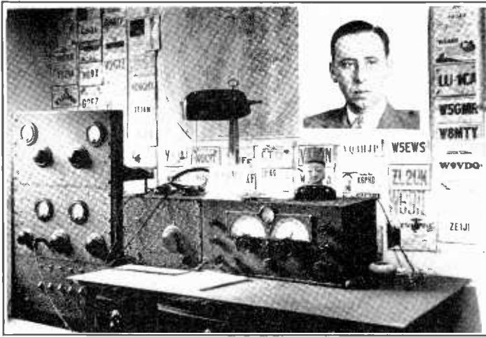
O. C. Miller, XU8MI, Shanghai, China. Transmitter uses a pair of 35T's with 400 watts input.
