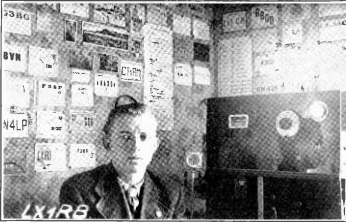
LX1RB, owned by R. Biltgen of Esch-Sur-Alzette, Luxembourg. The rig is a 6L6 electron coupled with 30 watts input. Antenna is a half-wave Hertz. Receiver is a two-tube home-built affair. LX1RB is usually on 14375 with a T8 signal.
